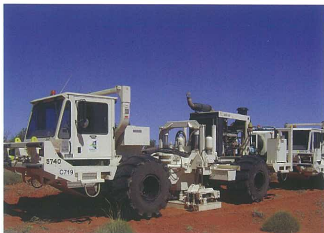
Fig 2. Three Vibroseis trucks are used for a seismic survey
